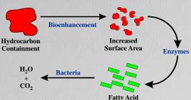
The microbes use a process of extracellular and intracellular enzyme production in which enzymes are excreted from the microbial cell. The microbes secrete various enzymes that begin the process of cleavage and digestion of the hydrocarbons. The enzymes chop the long-chains of the hydrocarbons into two carbon units which are used as a source of food for the microbes to reproduce.
